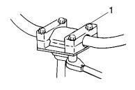
4. Torque the front two bolts to 10-12 ft. lbs. (14-17 Nm), then torque the rear two bolts. A gap of up to 1/8" (3 mm) will remain at the rear bolts.
